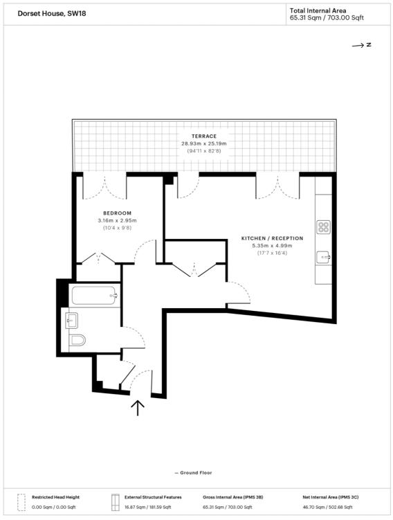
Spec floor plan captured for JLL, Nine Elms on 21/06/2018 using 165,093,397 laser scan points, accurate to +/- 3cm. Produced in accordance with Royal Institution of Chartered Surveyors Property Measurement Standards, incorporating International Property Measurement Standard (IPMS). If you intend to rely on any measurement in a transaction you should perform your own checks. Plot/Gardens illustrative only and excluded from all area
